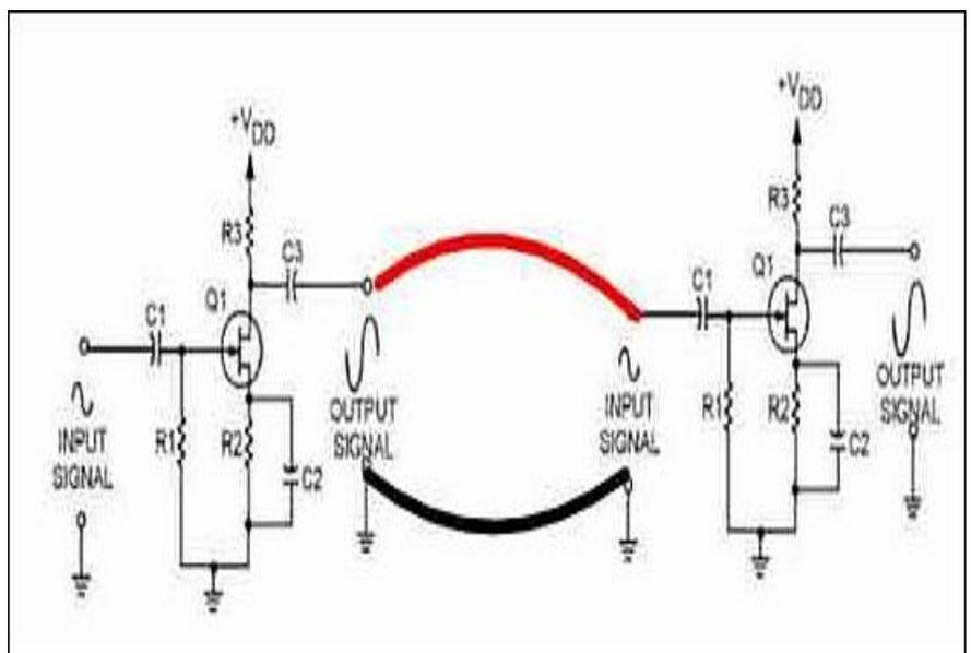
The two conductors, though, are in close proximity to each other, so as the electrical energy flows through the signal conductor noise is induced into neutral conductor and vice versa. If coupling feedback effects, ie induction processes, occur between the signal and neutral conductors due to electrical noise, capacitive and inductive reactive effects, impedance interaction effects, and/or ground flow issues then an impeded *effective signal flow* will result.
